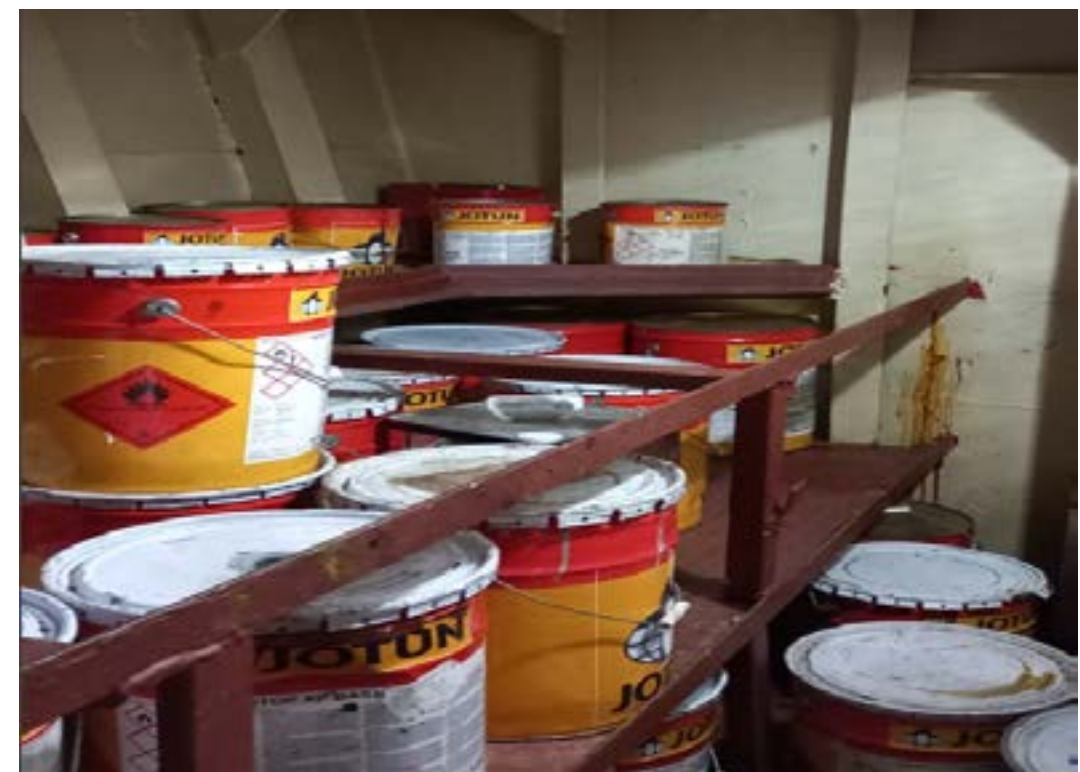
Unlashed paints in paint room
