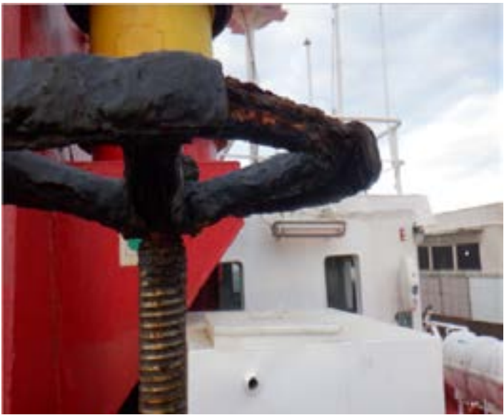
Damaged/heavily corroded ventilation handle
