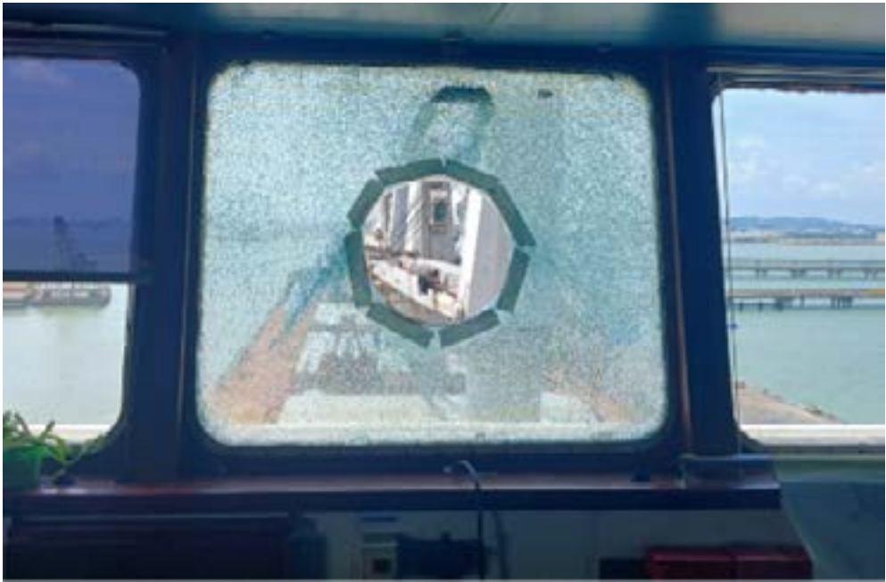
Broken Bridge Window
