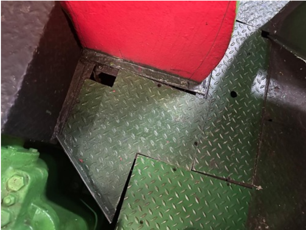
Non-secured bilge floor gratings
