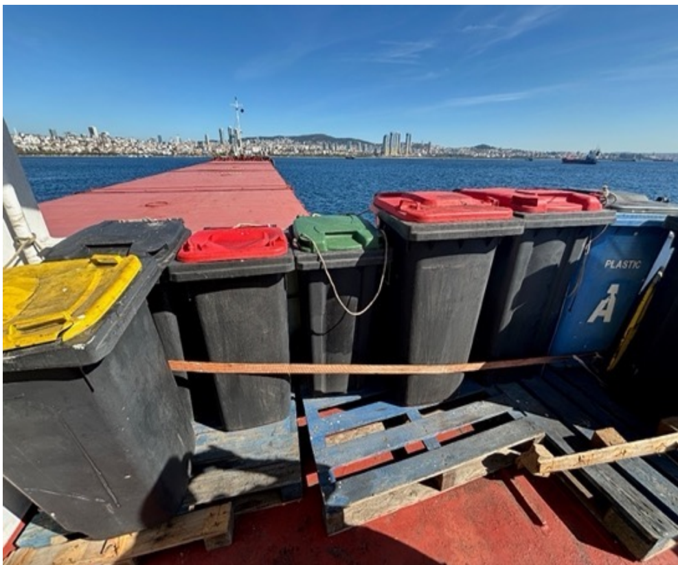
Garbage receptacles are not identified
