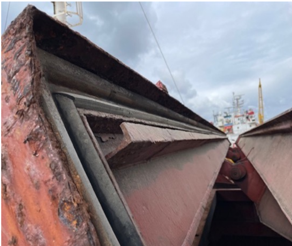
Corroded hatch cover and gaskets
