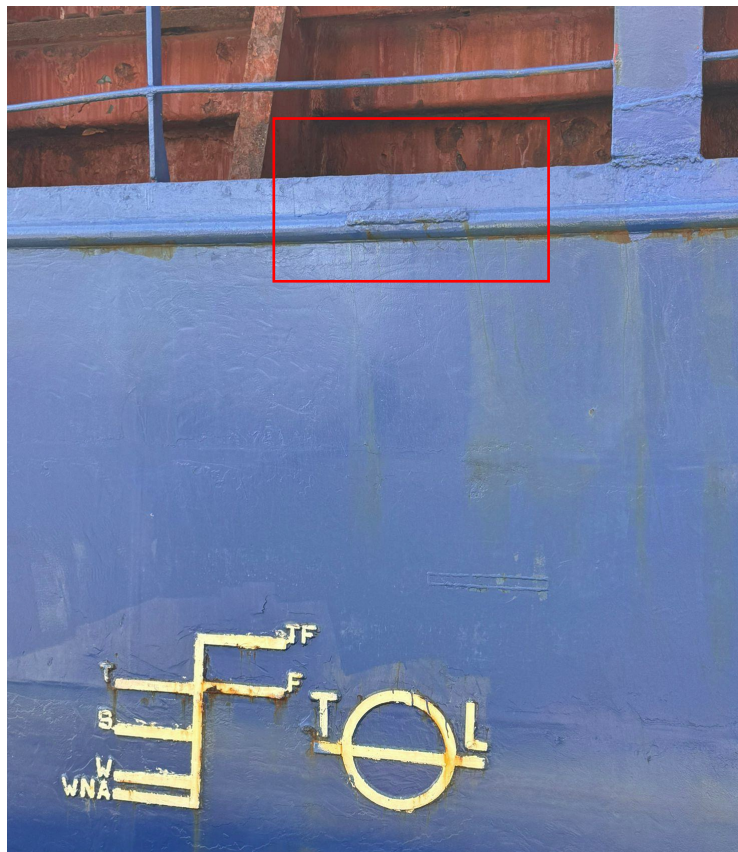
Not-painted deck line
