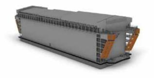
Dimensions(m): 105 x 25.1 x 19.9Lifting Capacity: 3.000 TonGenerator: 4 x 750 kWConstruction Shipyard: HİCRİ ERCİLİ<br/>Shipyard
