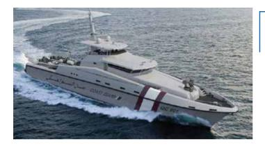
Dimensions *(m)* Main Engine Max. Speed *(kts)* Construction Shipyard Ship's Name Quantity : 47.9 x 8.78 x 1.78 : 3 x 2240 kW : 36 : ARES Shipyard : QC 901 - QC 902 : 2
