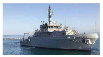
Dimensions(m): 41.20 × 9.55 × 4.5Main Engine: 2 × 1000 kWMax. Speed (kts): 12Construction Shipyard: TURKMENBASHI<br/>Shipyard
