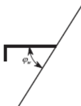
Figure 14 : Angle between stiffener web and attached plating
