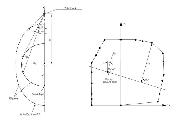
= resulting acceleration (static and dynamic) in arbitrary direction  $\boldsymbol{\beta}$
