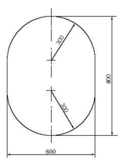
.3 Circular access openings in type-C cargo tanks should have diameters of not less than 600 mm.
