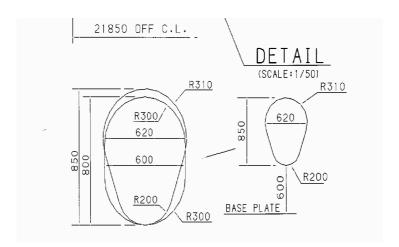
3. If a vertical opening is at a height of more than 600 mm steps and handgrips are to be provided. In such arrangements it is to be demonstrated that an injured person can be easily evacuated.
