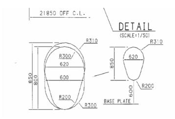
3. If a vertical opening is at a height of more than 600 mm steps and handgrips are to be provided. In such arrangements it is to be demonstrated that an injured person can be easily evacuated.
