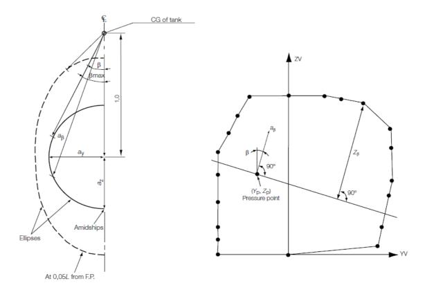
$a_{eta}$  = resulting acceleration (static and dynamic) in arbitrary direction eta
