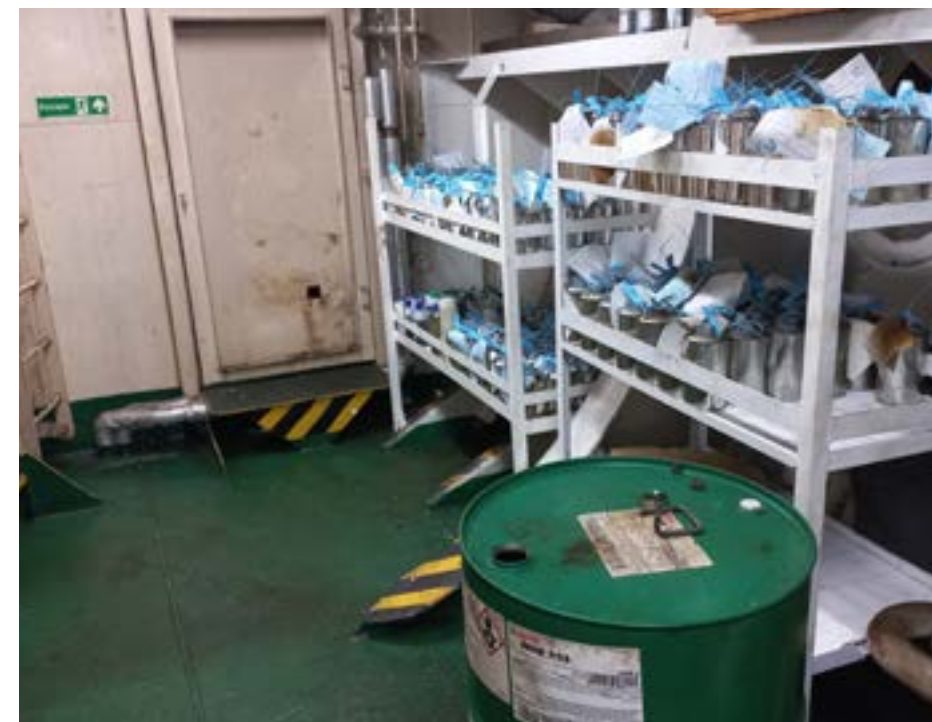
Bunker samples stored in steering gear room without MSDS
