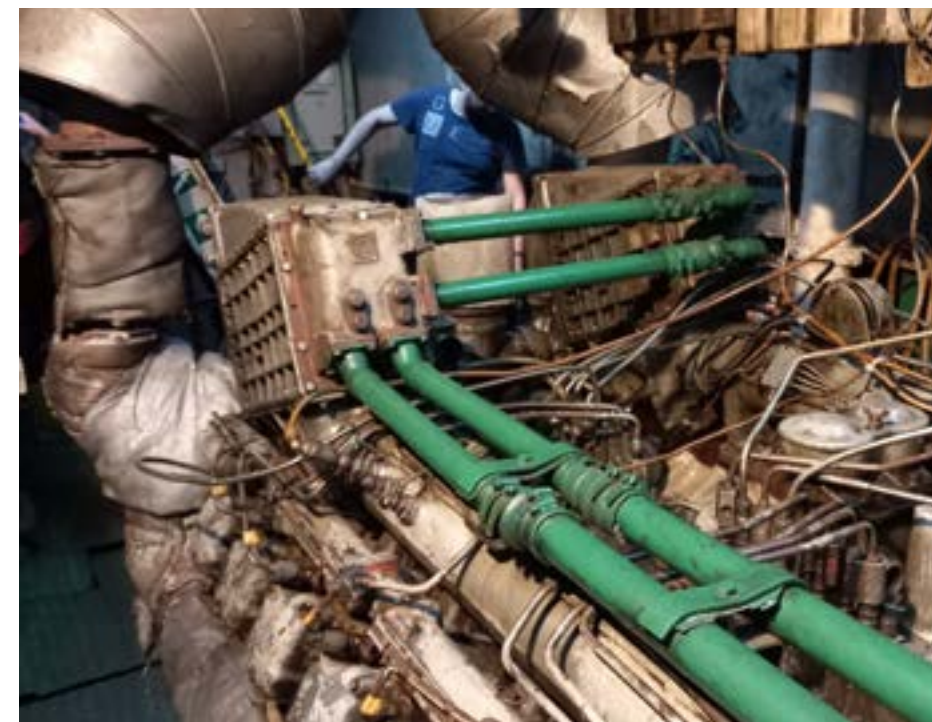
Unproper and missing exhaust insulation in main engine
