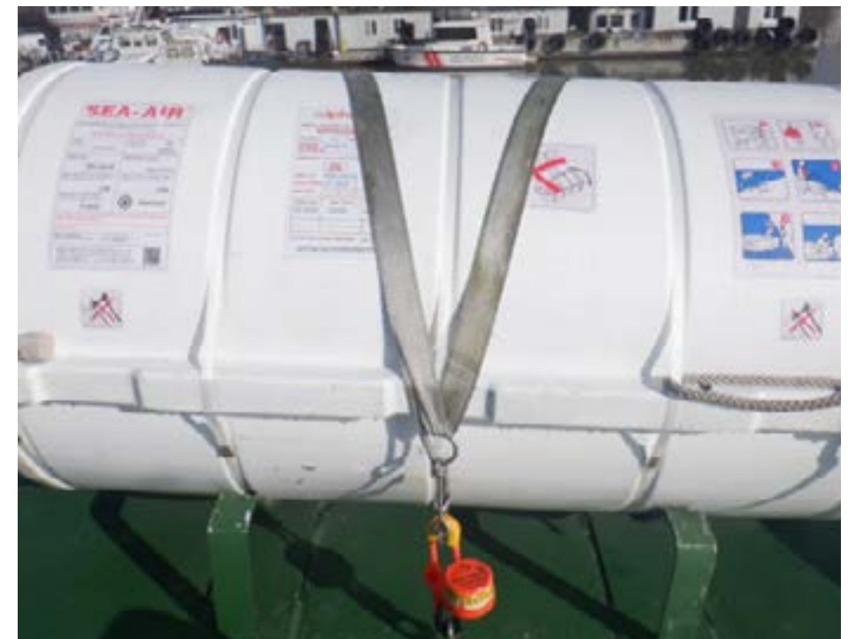
Liferaft missing weak-link connection
