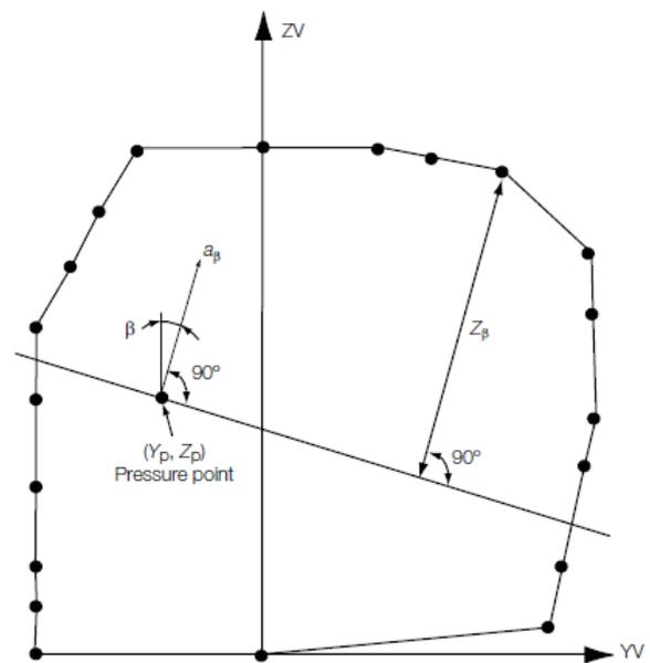
**Fig.2 Determination of internal pressure heads**
